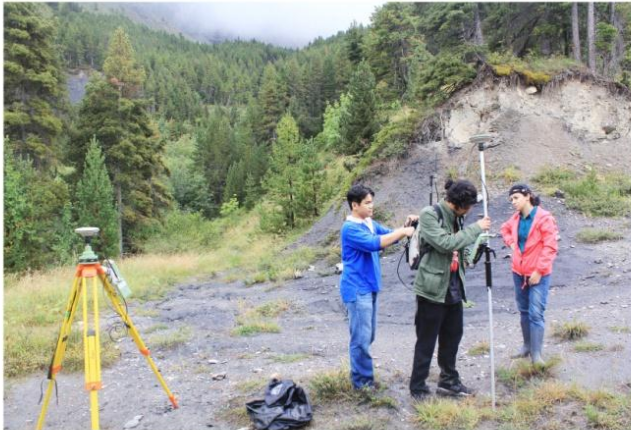
Setting base station and rover set for differential GPS
